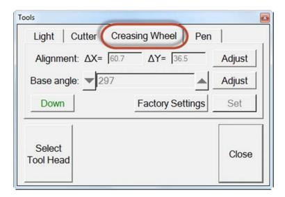
This menu defines two of the basic system features of the creasing wheel instrument – **Alignment** and **Base angle.**
