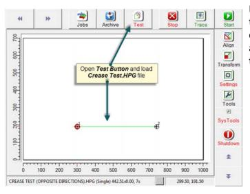
Put a sheet of paper on the vacuum table and start the vacuum. Align the drawing at a proper place on the work area. Press **Start** button and run the test file.
