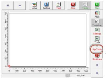
**System tools** tab is accessible only in System mode.
