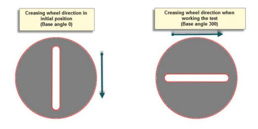
Setting the correct base angle value for each instrument requires the following steps:
