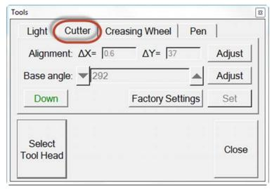
This menu defines two of the basic system features of the cutting instrument – *Alignment* and *Base angle*.
