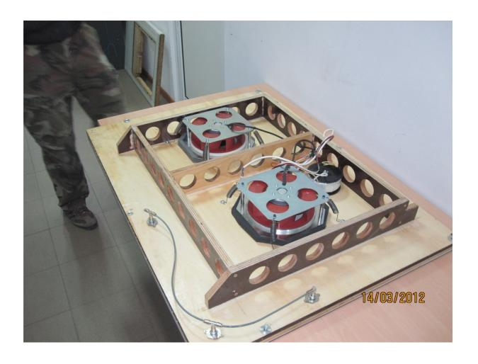
12. Remove the 8 springs fixing the fans, by disconnecting their upper sides from the fan plate
