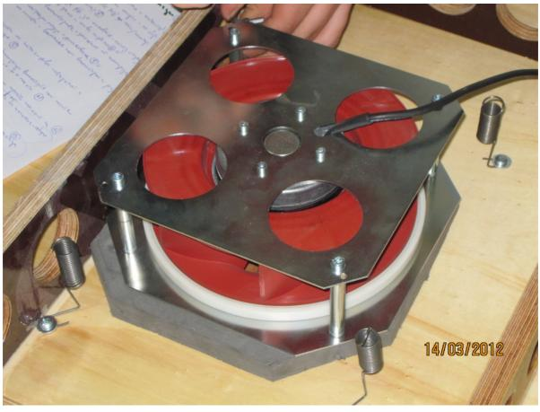
13. Clear carefully the fan rotors and stators from all mechanical objects, dirt etc. as result from their functioning.
