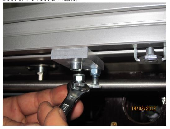
Pay attention not to move the leveling nuts that are fixing the correct level of the vacuum table
