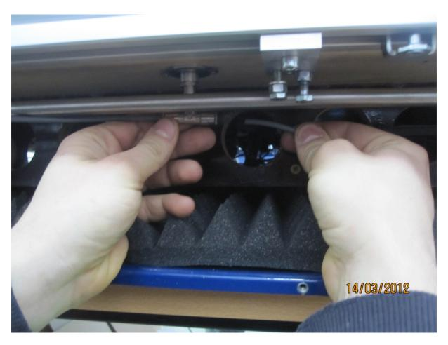
8. Unscrew the middle support M6 screws in the back and front sides of the vacuum table.
