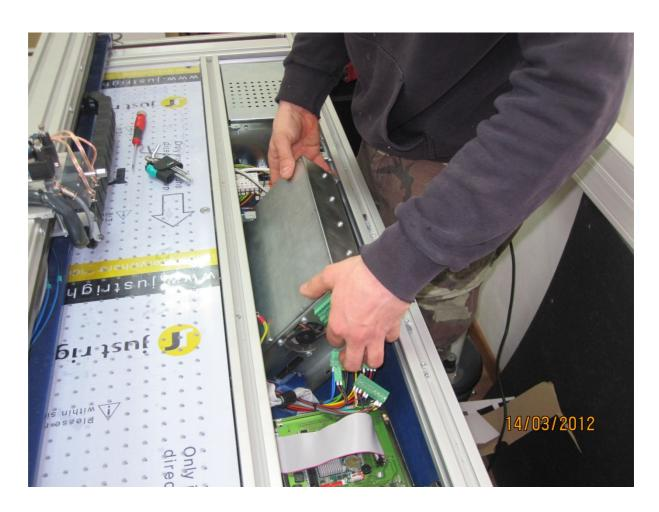
7. Disconnect the air pipes for the fixation pins under the front side of the vacuum table
