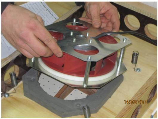
14. Unscrew the M5 bolts attaching the top plate to the fan
