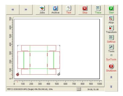
The name of the current job (Fefco 0330 body.hpg in this case), the type of the file – single or double, the dimensions of the file (496.50x340.60) and the estimated time for completing the job (104s) are displayed in the lower left area of the main screen.
