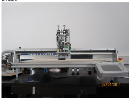
3. Move by hand the X bar in the most rear position (axis Y max)
